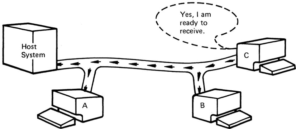
3. Having answered yes, terminal C is ready to receive the data. The host system sends the data and only terminal C processes it (terminals A and B ignore the data):
