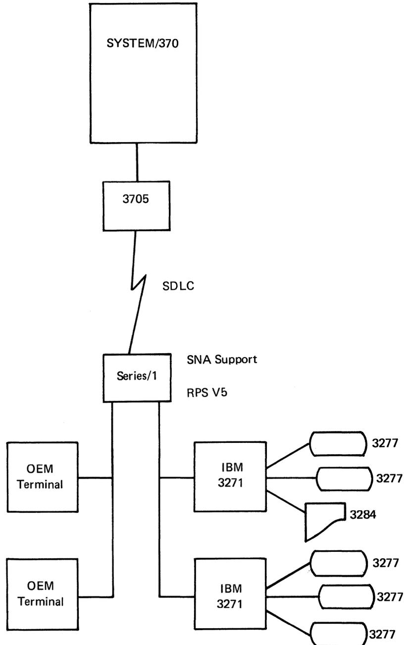
This configuration shows a Series/1 using SNA/SDLC to communicate with a System/370 and support IBM and OEM terminals at the same time.
