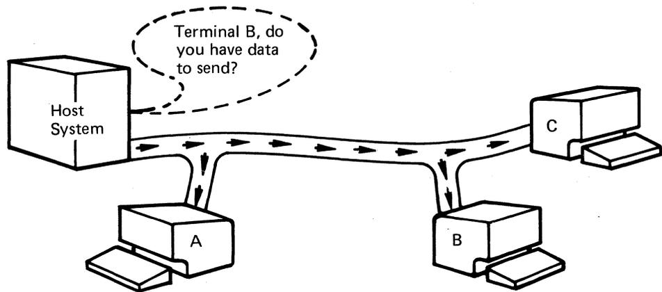
4. This time only terminal B answers. Terminal B is ready and has a message for the host system (terminals A and C ignore the data and the response):
