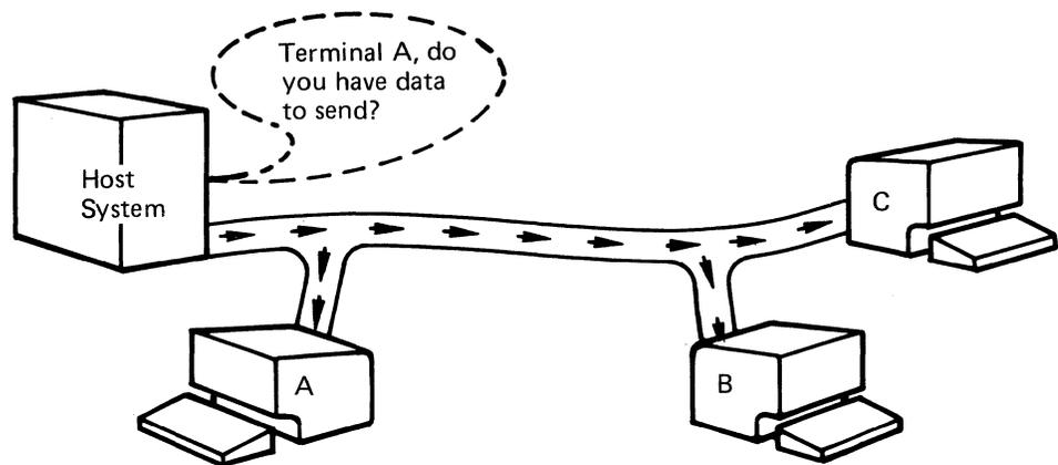
2. Although all terminals on the line receive the address for terminal A, only terminal A answers. (Terminals B and C receive the response but ignore it.) If terminal A does not have data to send or is not ready to send data, it indicates this in its response:
