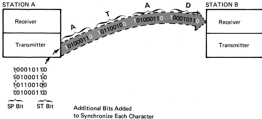
The 0 bit in the beginning of each character is called a start (ST) bit. The 1 bit at the end is called a stop (SP) bit. The receiving station recognizes these additional bits as the beginning and end of each character. The start and stop bits of each character keep the clocks in sync for that character.
