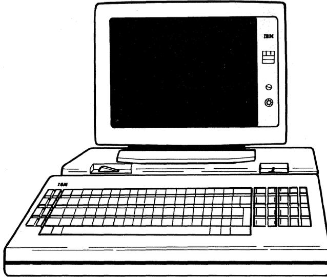
The IBM 3101 Display Terminal is an adjustable display station that allows interactive communications using ASCII. The 3101 is a keyboard display with a screen format of 1920 characters. Characters are presented in a 7 x 14 dot matrix within a 9 x 16 dot matrix.
