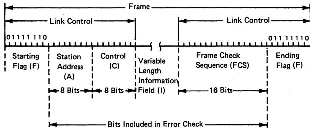
**Flag (F):** The beginning and end of each frame is indicated by a series of bits (01111110) called a flag. In some machines, the ending flag of one frame can be used as the starting flag of the next frame.
