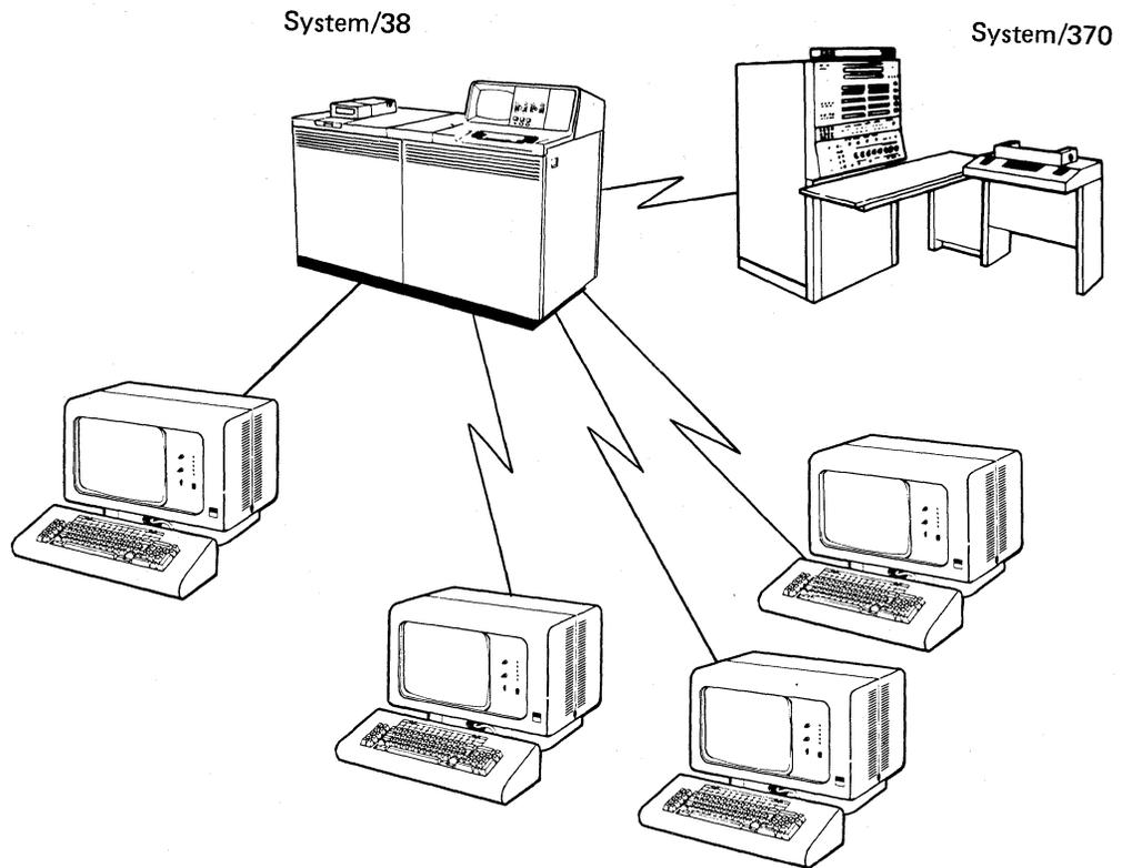
Using BSC, RJEF communicates with host systems over a point-to-point switched or nonswitched communications line.
