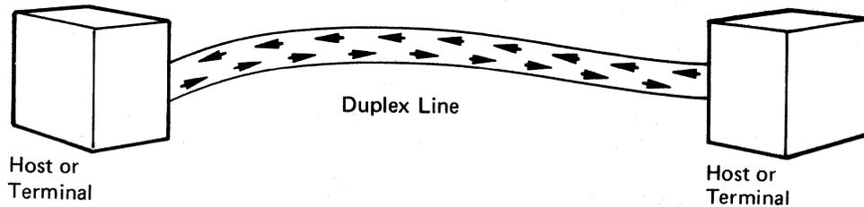
Half-duplex transmission is data transmission in both directions but not at the same time. Examples of half-duplex data transmission follow. In the first example, a host is the transmitter and the terminal is the receiver. In the second example, the terminal is the transmitter and the host is the receiver.
