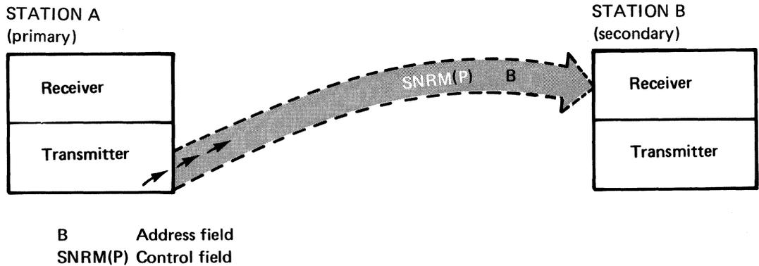
**Note:** The flags and check field are always transmitted with each frame, although they are not shown in the example. Also, the address field always contains the address of the secondary station.
