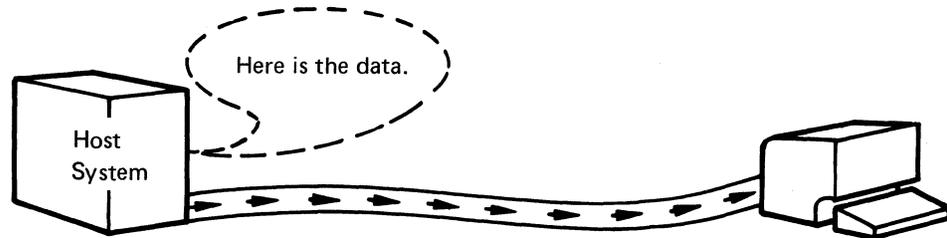
The terminal normally indicates to the host whether or not the data was received correctly.
