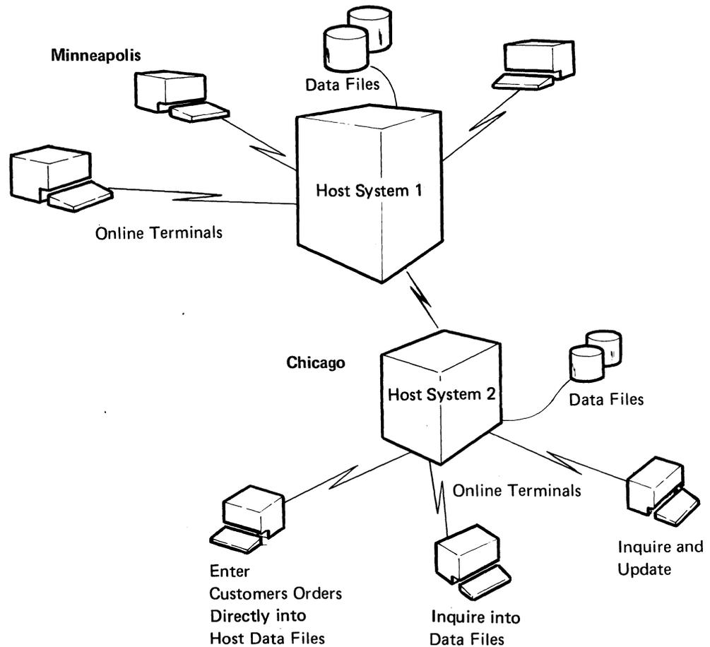
In this configuration, host system 2 is a host for its terminals and is a terminal for host system 1. Host system 2 performs the following:
