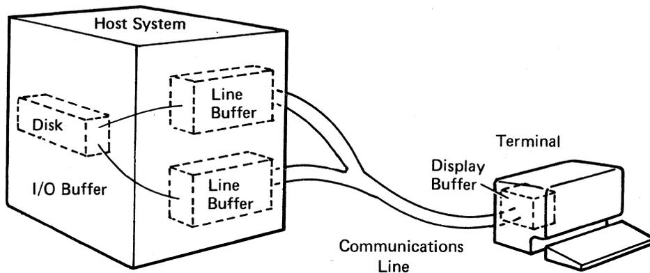
Two line buffers are used to store data that is being transmitted to the line or being received from the line. During a transmit operation, data can be transmitted from one line buffer while data to be transmitted next is placed in the other line buffer. During a receive operation, data from the line can be stored in one line buffer while previously received data, stored in the other line buffer, is processed.
