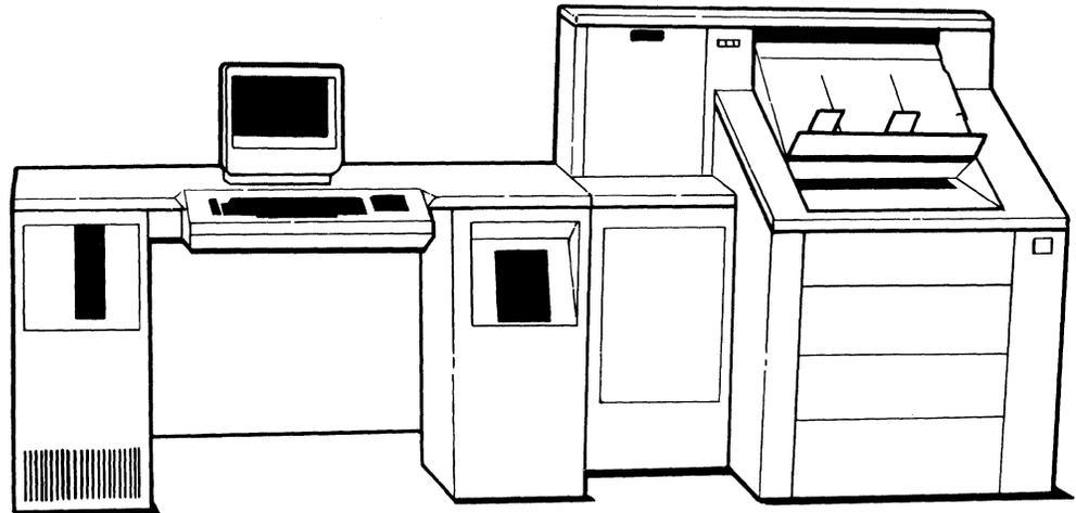
The IBM Office System 6 (OS/6) is a text processing system that allows you to enter, edit, and format text, and process and maintain records.
