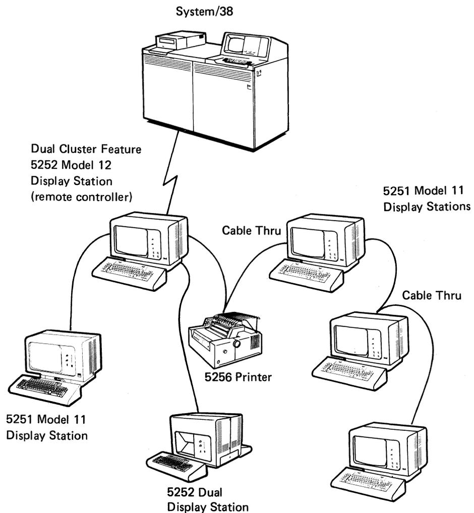
The following shows a typical System/38 configuration with remote work stations. In this illustration, the System/38 is installed at a company's main office and plant in Chicago. The company also has sales offices in New York, Milwaukee, and Madison.
