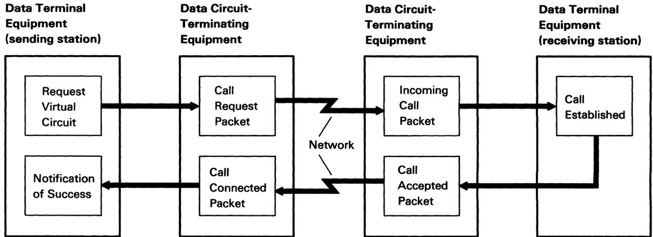
The calling station sends a call request packet to the remote location. At the receiving station, the incoming call packet is received and a call accepted packet is returned to the network. At the calling DTE, a call connected packet is returned, showing that the switched virtual circuit has been established.
