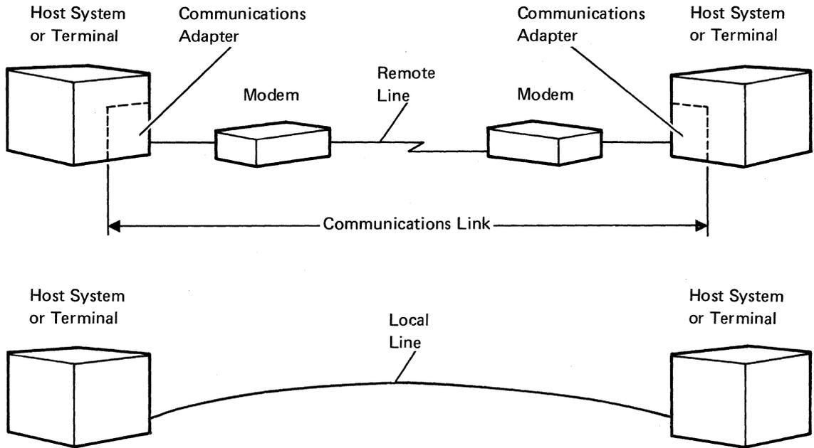
The communications link is the path from a computer to a terminal or another computer. The communications link includes the lines, modems (when used), and communications-controlling portions (programs and devices) of the terminal or other computer.
