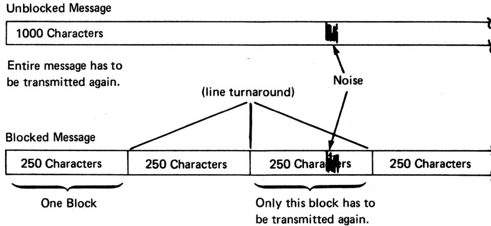
In this example, the transmitting station sending a blocked message only has to send 250 characters again instead of the entire message. The block size used depends on how the data communications system is used, the transmission speed, and the condition of the line. (Line conditioning occurs when certain devices are added to the line to improve the data signal.)
