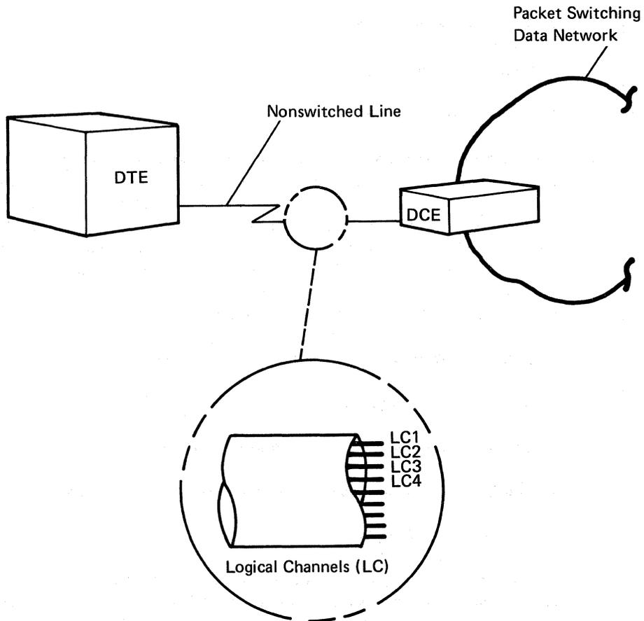
Logical channel numbers are assigned to a virtual circuit only across the DTE and the DCE connection. In this example, logical channel numbers 1, 2, 3, and 4 are assigned to the line between your DTE and DCE. (Logical channel numbers would also be assigned to the link between the remote DTEs you will communicate with and their associated DCE.)
