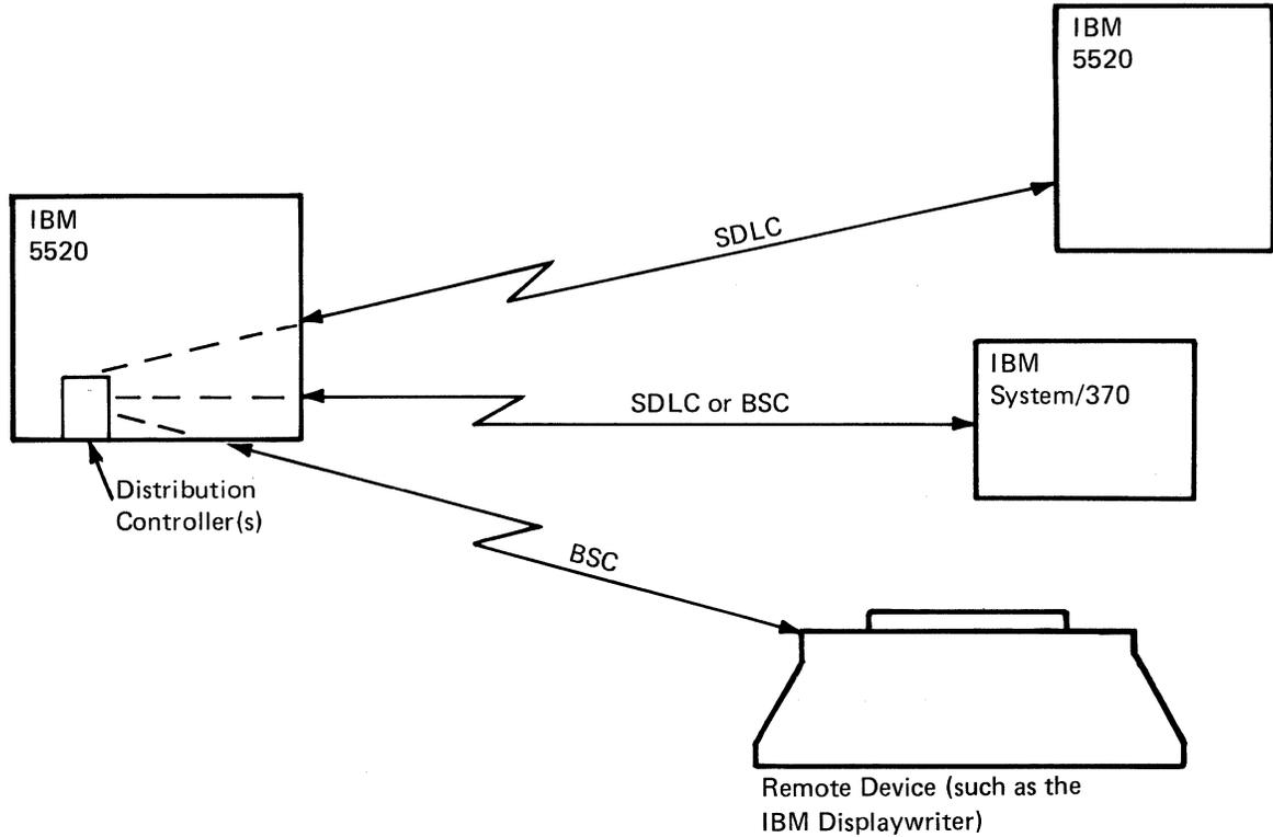
The following illustration shows an IBM 5520 communicating with application programs on a System/370, using BTAM or TCAM.
