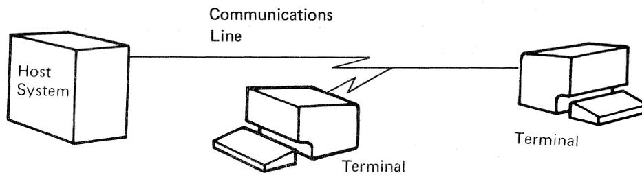
Three stations, a host and two terminals, are now connected to one line. Multipoint lines are usually nonswitched lines.
