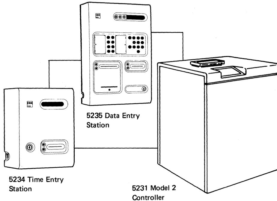
The IBM 5230 Data Collection System can be used to enter data at entry stations located in work areas. The 5234 Time Entry Station is for badge entry only; the 5235 Data Entry Station accepts data from cards, keyboards, and badges. The entry stations are attached to the 5231 controller.
