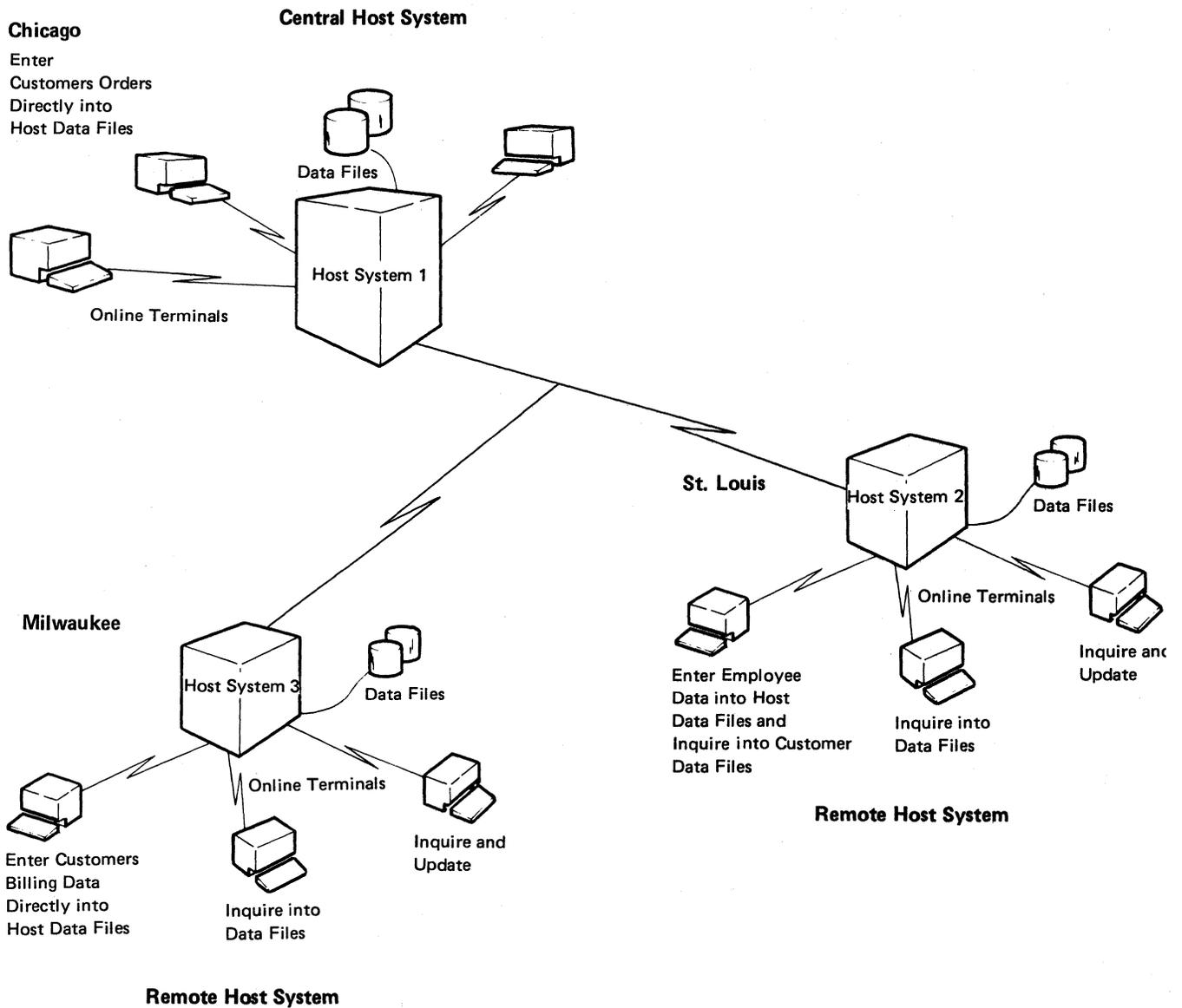
This illustration shows a distributed data processing configuration. In the configuration, remote systems and terminals are connected to a central processing unit, host system 1.
