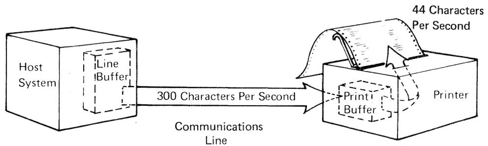
The data can be sent to the printer at line speed (300 characters per second), stored in the print buffer, then printed at printer speed (44 characters per second).
