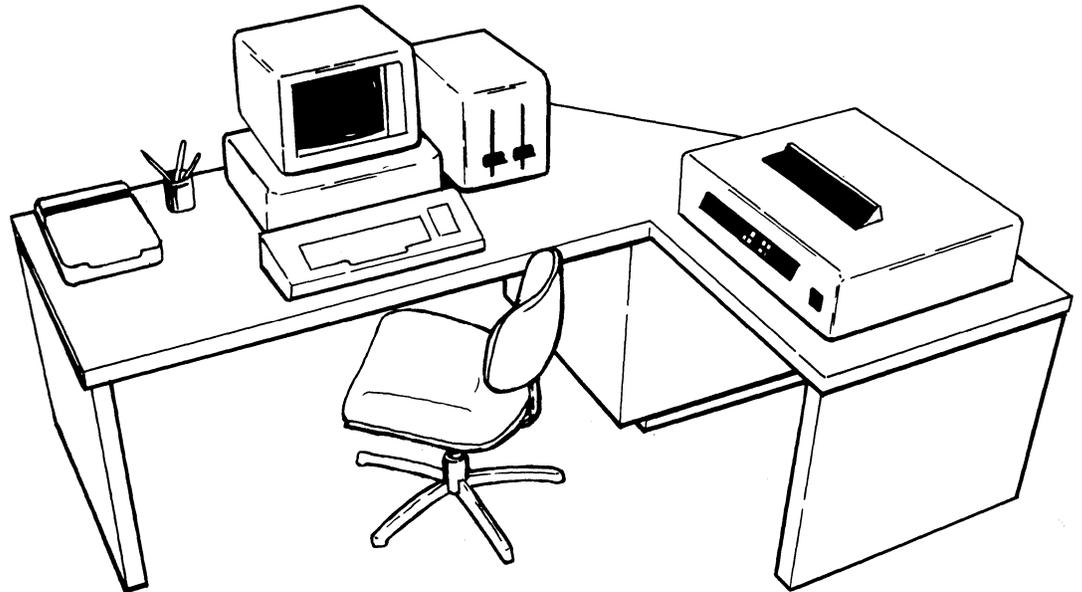
The IBM Displaywriter System is a diskette-based text processor that allows you to create and edit text, create, revise, display, and print charts, and send and receive information over communications lines from other office equipment and computers.
