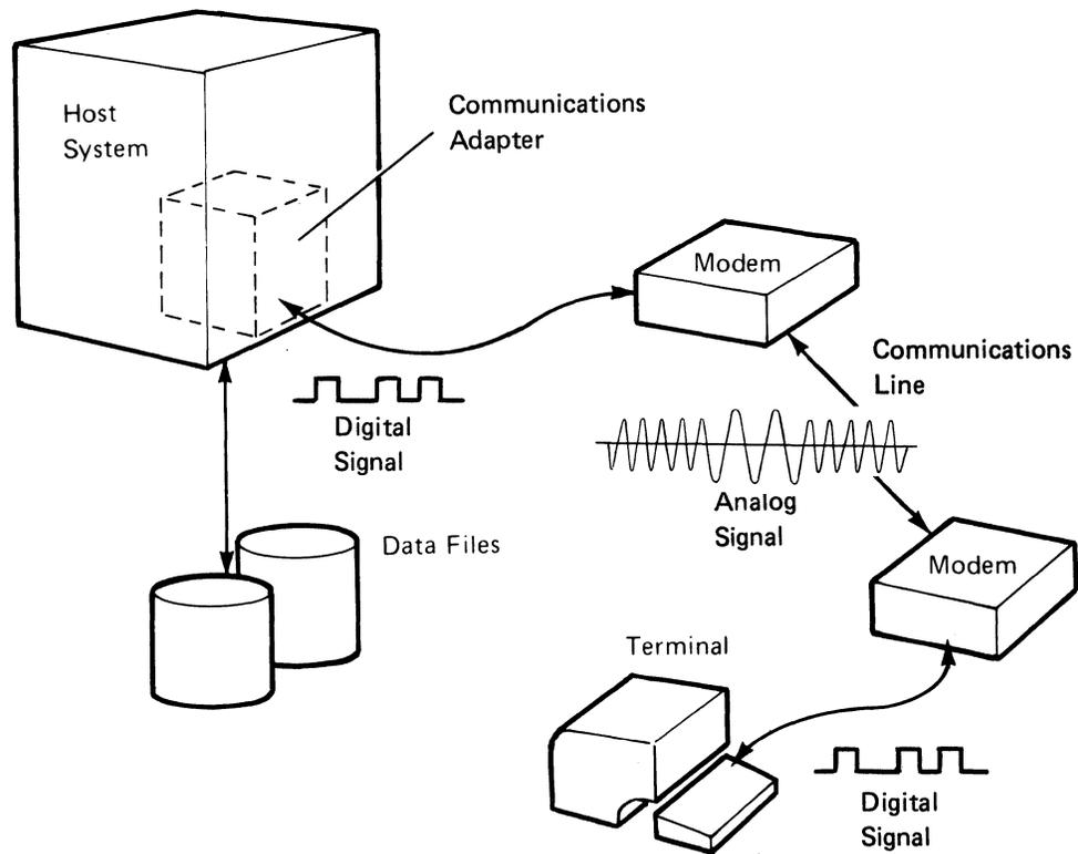
Modems may also be called data sets, data pumps, or line adapters. They can be external to, or enclosed in (integrated) a computer or terminal. There are a variety of modems available, some of which perform functions in addition to converting signals. Some of the additional functions (usually optional) that are available with modems are:
