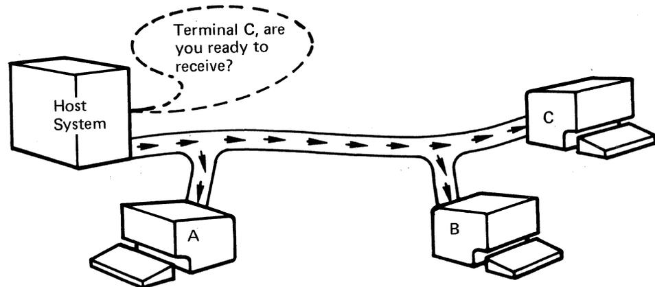
2. Only terminal C responds to the address sent by the host (the other terminals on the line receive the address sent by the host and the response sent by terminal C but ignore both):
