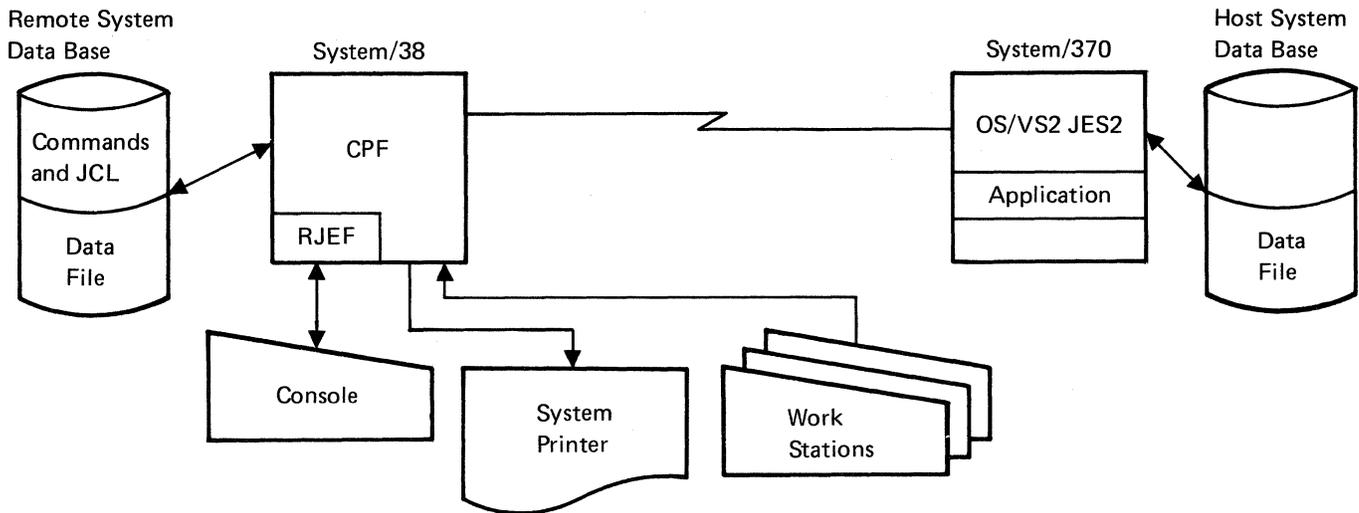
RJEF uses the BSC or SNA/SDLC support provided by the System/38 Control Program Facility (CPF) to transmit data and maintain line control. The Remote Terminal Access Method (RTAM) is used to communicate with host systems using BSC while the Virtual Telecommunications Access Method (VTAM) is used to communicate with host systems using SNA. All data is transmitted using the EBCDIC transmission code.
