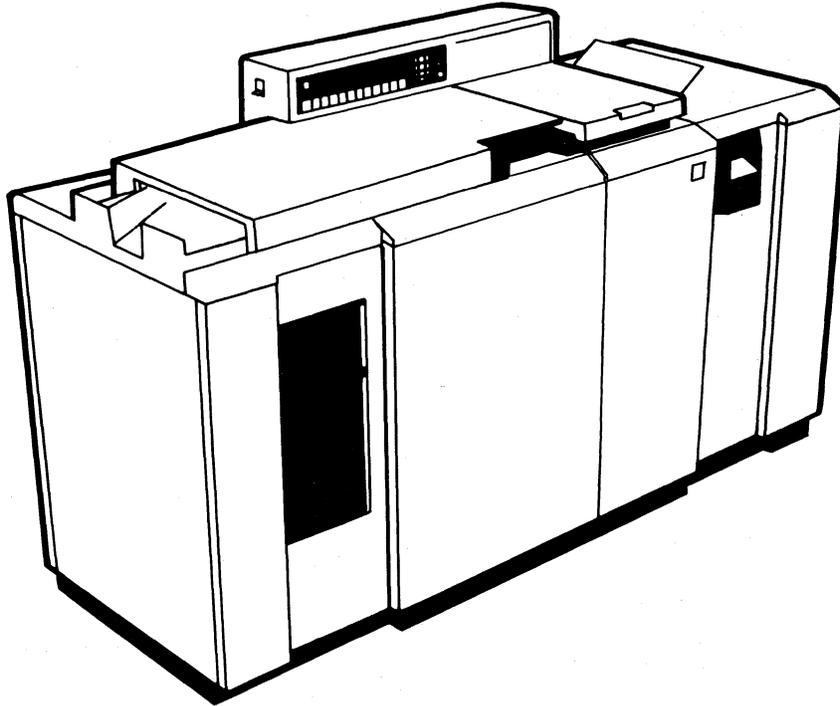
The IBM 6670 Information Distributor is a laser printer/copier that prints, records, sends, and receives information using communications lines. Documents are automatically formatted during printing.
