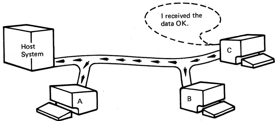
5. The host system then sends more data, or indicates the end of transmission (the end of transmission indicates that terminal C is no longer selected and the line is now available):
