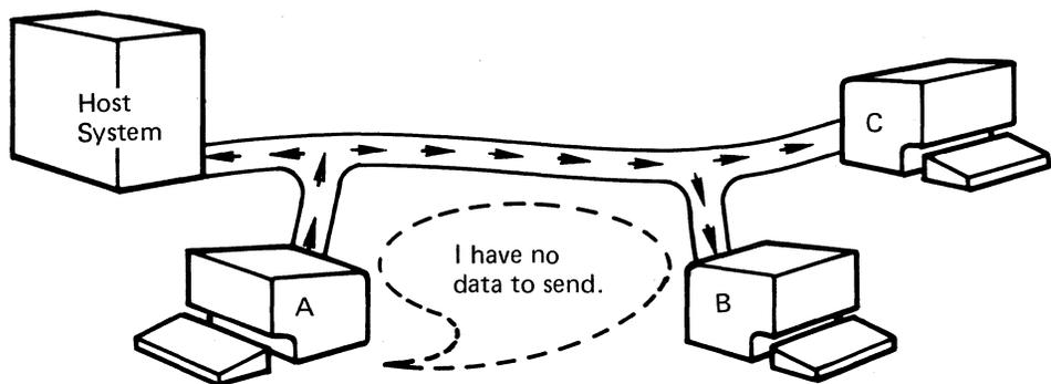
3. Since terminal A does not have data to send, the host system polls terminal B:
