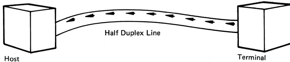
The terms 2-wire and 4-wire are sometimes used to mean half duplex and duplex; however, the number of wires in the communications line is not related to half duplex or duplex ability. See *Transmission Methods* later in this chapter for more information.
