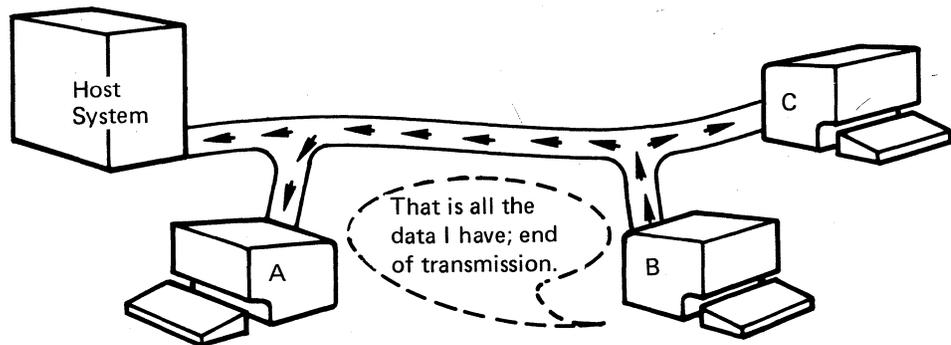
Terminals do not have to be polled in sequence. A polling list can usually be set up for the most efficient operation. If a terminal is seldom used, it does not have to be polled as often as a more active terminal. For example, if terminal C is used less frequently than terminals A and B, the polling list could look like this:
