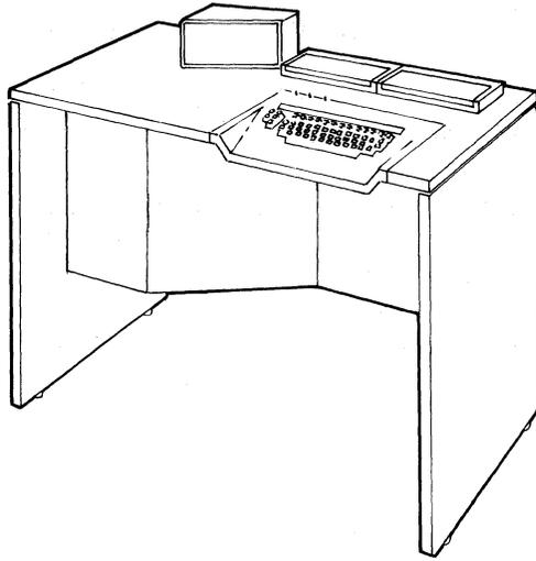
The IBM 3741 Data Station or 3741 Programmable Work Station can be used to enter and store data on diskettes for later transmission to a host system.
