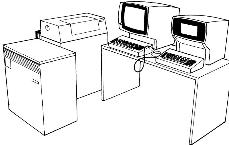
The IBM 3270 Information Display System consists of a display station (display screen and keyboard), a printer, and a control unit. The display system offers a choice of display sizes (with or without color), keyboard layouts, and printer speeds.
