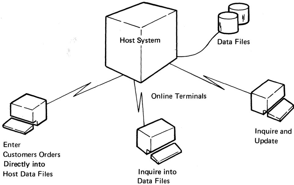
With this system, customer orders can be entered directly into host system files from a remote terminal. At the same time, other terminals can be used to inquire into and/or update host system files. In this system, data is received and processed and is ready to use immediately by the host or terminals. This is called interactive communications or realtime data processing.
