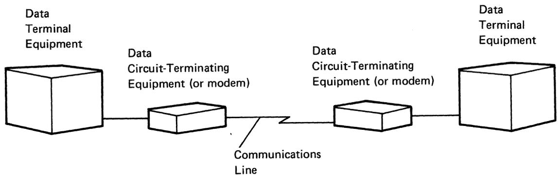
Several words are used to describe the electrical path between data processing devices in a data communications configuration: communications channel, communications lines, communications facility, and communications link. In this manual, the word *line* is used to describe all of the equipment that transmits the data from one modem to the other modem (remote line) or from one device to the other device (local line) as shown:
