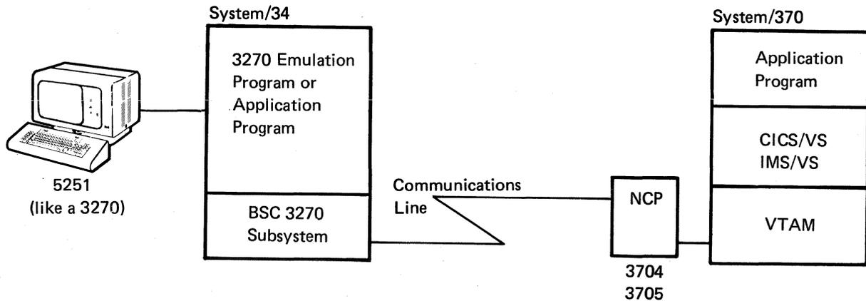
Because a System/34 or a System/36 appears as a remote 3277 Display Station, data sent by the host system that would have been displayed on a 3277 display screen is used instead to satisfy a System/34 or a System/36 application program input operation. Conversely, data from a System/34 or a System/36 application program output operation appears to the remote system as if entered from a 3277 Display Station.
