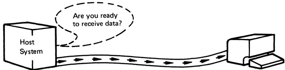
2. The terminal responds by indicating its status to the host. For example, a terminal might indicate that it is turned on, signed onto, and ready to receive data:
