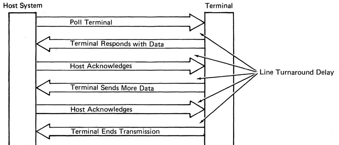
If a duplex line is used, the modems and network equipment are always ready to transmit and receive, and the line turnaround time is minimal.
