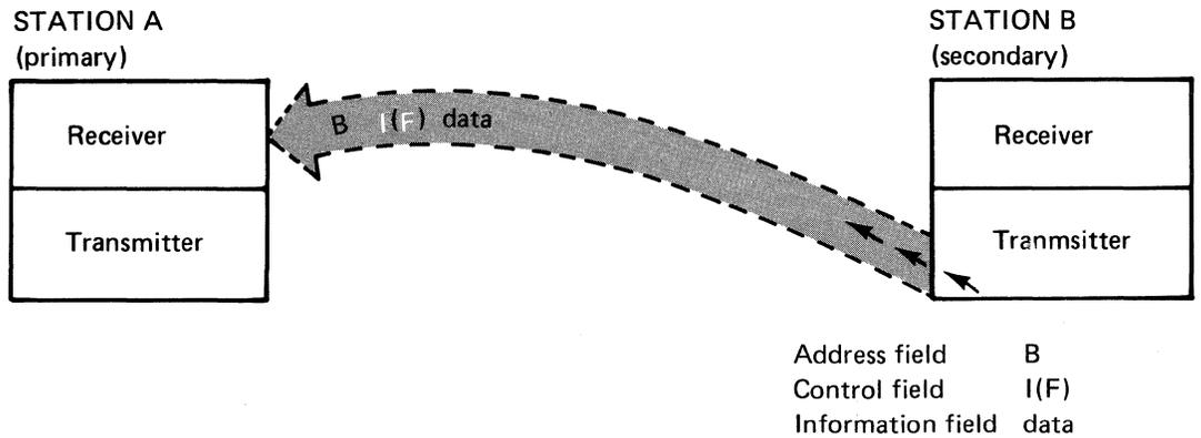
Station A acknowledges receiving the information frame with a receive ready (RR) command (the poll bit (P) is on to allow station B to send):
