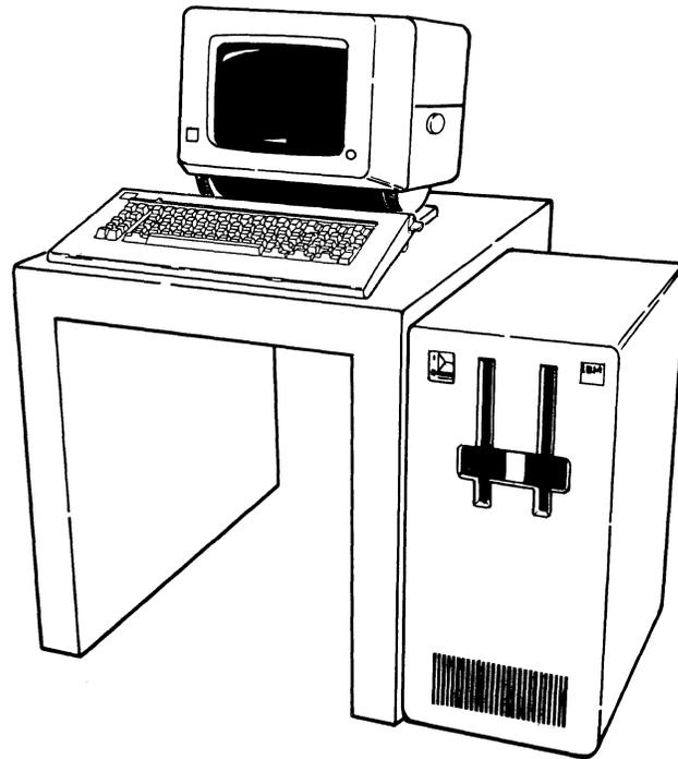
The IBM System/23 Datamaster is a small general purpose computer that uses a communications feature to communicate with other systems at other locations, or with other System/23s. The System/23 consists of the following:
