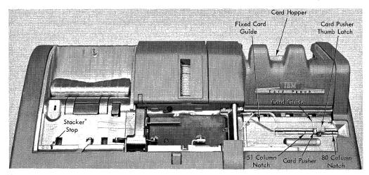
Figure 20. Variable-Length Card Feed Device
