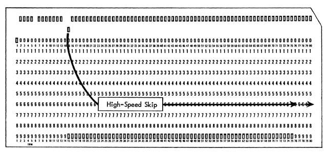
Figure 19. Program Card Showing High-Speed Skip Punching
