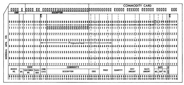
Figure 15. Error Correction—Partially Prepunched Cards
