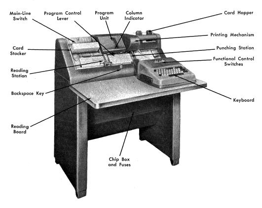
Figure 4. IBM 26 Operating Features
