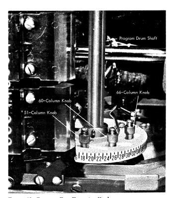
Figure 22. Program Cam Extension Knobs (80-Column Card Setting)
