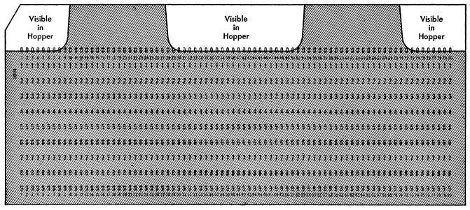
Figure 5. Card Visibility in the Card Hopper
