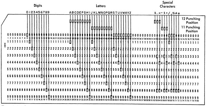
Figure 2. Punching Positions in Card
