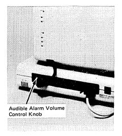
Figure 1-3. Audible Alarm Volume Control Knob (rear view of 3101)
