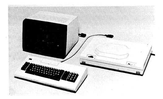
Figure 1-4. 3101 Display Terminal-Separated Work-Station Elements
