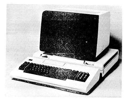
Figure 1-5. 3101 Display Terminal-Connected Work-Station Elements
