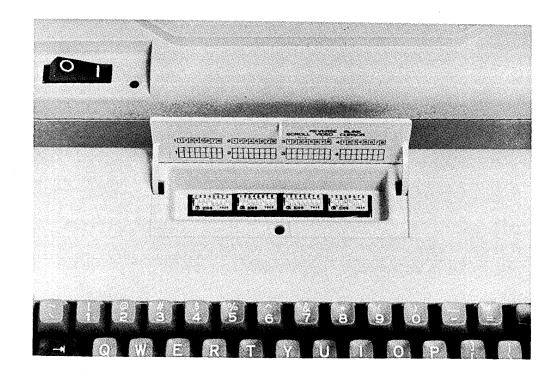
Figure 1-6. Setup Switches
