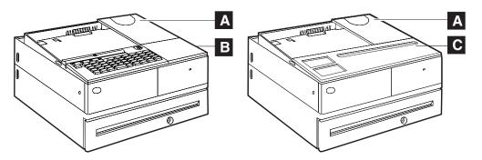
Figure 5. Installed filler panels for displays and keyboards
