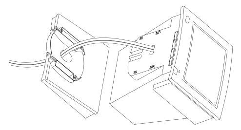
Figure 31. Location of the power cord and video cable for a wedge-mounted monochrome CRT
