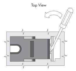
Figure 12. Removing and replacing the slide latches
