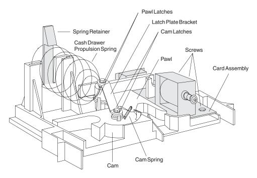
Figure 18. Cash drawer latch and sensor assembly
