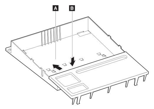
Figure 8. Installing the keyboard replacement filler panel
