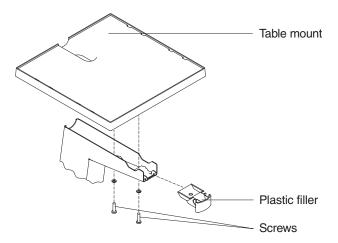
Figure 34. Table mount attached to post mount
