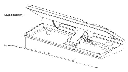
Figure 50. Removing the keypad assembly
