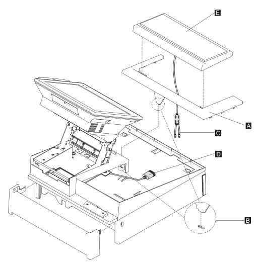
Figure 45. Removing the keyboard from the integration tray
