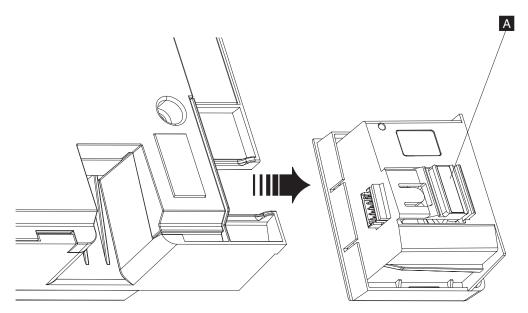
Figure 43. Removing the keylock or biometric device from a modular keyboard
