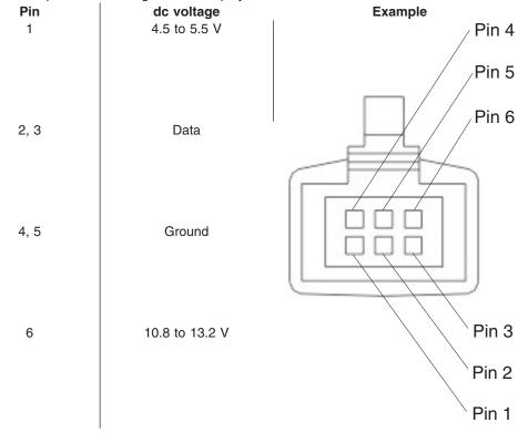
Table 9 describes the pins and provides an example of the USB cable connector on the device end of a keyboard or LCD cable.
