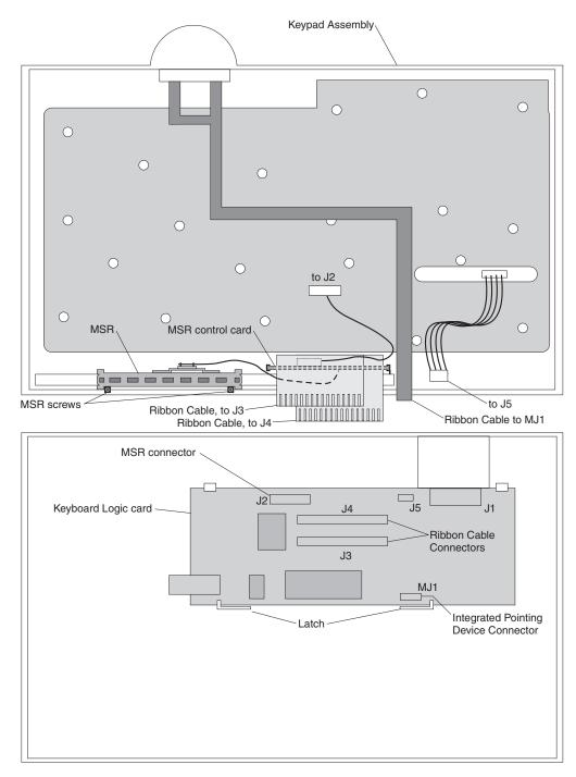
Figure 47. CANPOS keypad assembly with MSR
