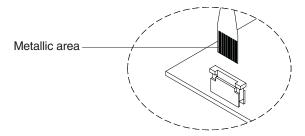
Figure 52. Removing the flexible cable from the connector holder
