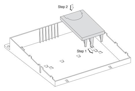
Figure 6. Installing the display filler panel
