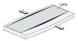
Figure 24. Removing the lens
