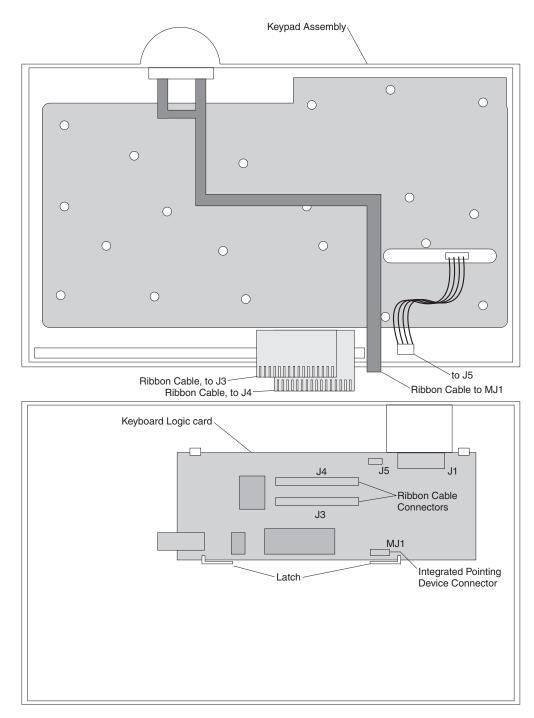
Figure 46. CANPOS keypad assembly without MSR
