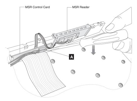
Figure 48. Removing the MSR control card
