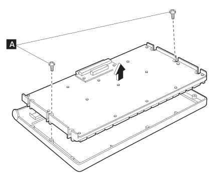
Figure 64. Removing the screws
