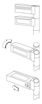
Figure 25. Disassembling the display
