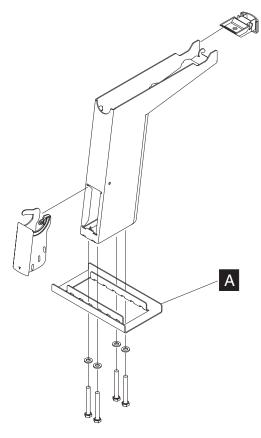
Figure 33. Attaching CRT to the counter
