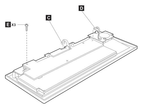
Figure 57. USB keyboard-V components - part 2
