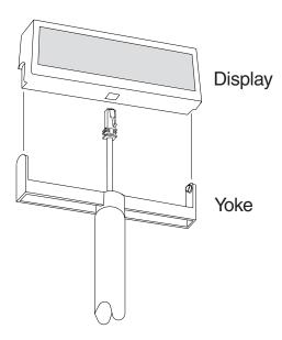
Figure 22. Removing and replacing the display
