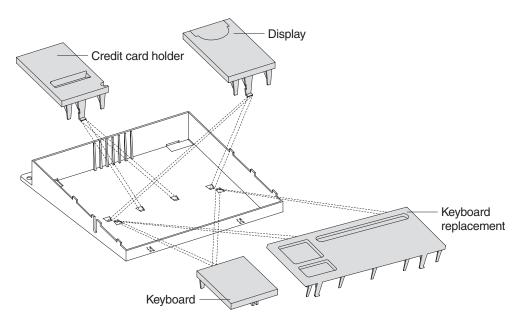
Figure 4. Mounting locations of the filler panels
