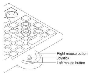
Figure 38. Example of a PS/2 ANPOS keyboard with integrated pointing device
