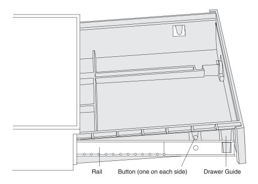
Figure 2. Removing and replacing a full-size cash drawer
