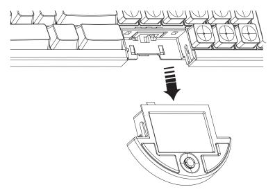
Figure 42. Removing the integrated pointing device from a modular keyboard
