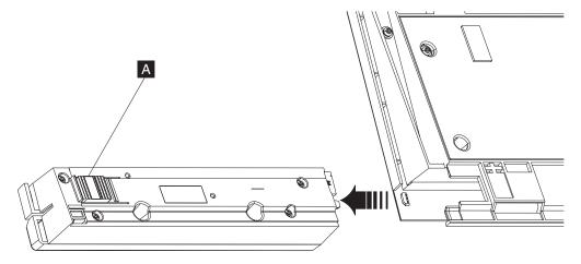
Figure 41. Removing the MSR from a modular keyboard
