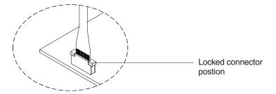
Figure 54. Locked connector position
