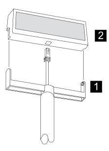
Figure 29. Removing and replacing the character/graphics display
