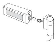
Figure 26. Disconnecting the display cable from the post
