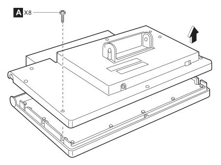
Figure 62. Removing the cover of the USB PLU keyboard/display
