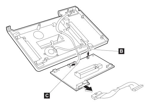
Figure 67. Disconnecting the connector to the LED assembly
