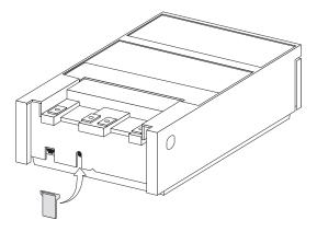
Figure 16. Removing the security clip (compact cash drawer)
