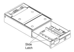
Figure 11. Removing and replacing the compact cash drawer
