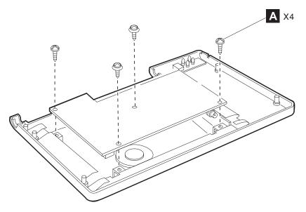
Figure 66. Removing the screws
