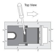
Figure 10. Releasing the drawer from the slide assembly
