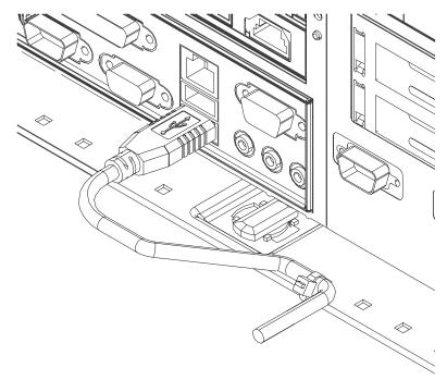
Figure 37. Securing the cable with cable ties
