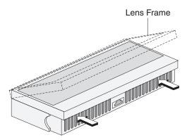
Figure 23. Removing the frame
