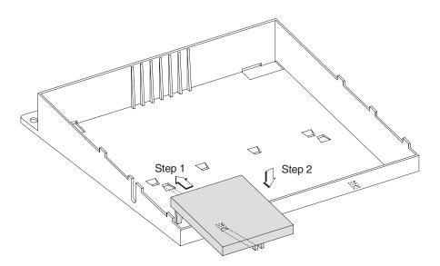
Figure 7. Installing the keyboard filler panel
