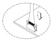
Figure 53. Inserting the flexible cable
