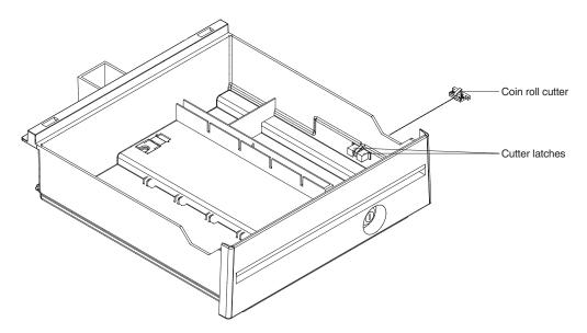
Figure 15. Removing the coin roll cutter
