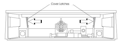
Figure 17. Removing and replacing the top cover
