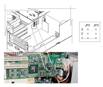
Figure 1. Setting the cash drawer using the jumper override
