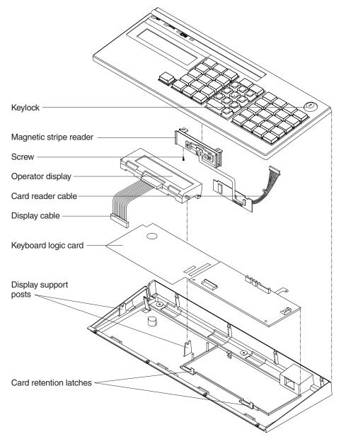
Figure 49. Removing keyboard components
