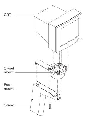
Figure 30. Post-mounted CRT
