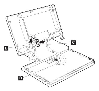
Figure 65. Disconnecting the connector, screws, and cables
