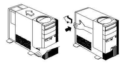
Slide the lock on the back of the unit to the "locked" icon to secure the cover to the chassis.
