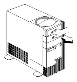
**NOTE:** Removing the system cover, exposes metal plates in front of each unpopulated drive bay. Push back and break-off these metal plates before installing additional drives.
