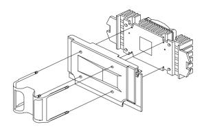
To remove the SECC2 type fan sink, use a screw driver to slide the fastener nodes outward to unlock the fan sink from the processor, then carefully remove the fan sink from the processor.
