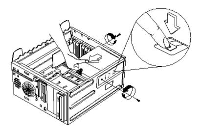
• Detach the power supply from the frame by removing it's four screws.
