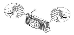
· Firmly hold the processor module and pull it out of the socket.
