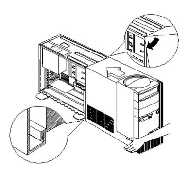
Slide back the cover until it fits into place. If the cover does not slide all the
