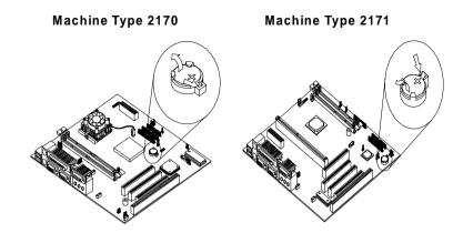
**IMPORTANT:** Make sure to insert the battery with the positive side facing up. A plus(+) sign indicates the positive side.
