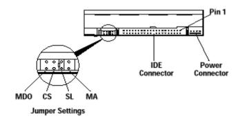
**NOTE:** Set the jumpers located on your LS-120 drive according to your system configuration. If you have two drives on a single IDE cable, make sure you set one of them as Master and the other as Slave.
