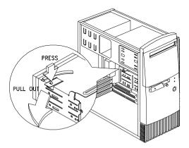
Remove the screws located on both sides of the drive and slide the drive out.
