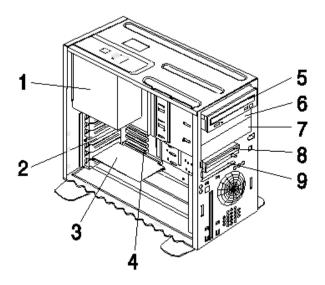
This computer system has five bays that can hold up to three 5.25-inch and two 3.5-inch drives. Additional devices can be installed in the empty bays.
