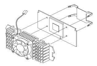
7. With the processor card golden fingers pointing downward, align the processor to the posts of the URM.
