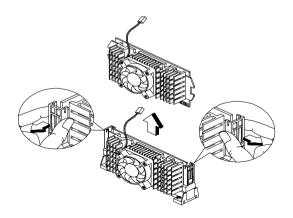
• Use a screw driver to push the four fastener tabs outward to unlock the heat sink from the processor, then carefully detach the heat sink from the processor.
