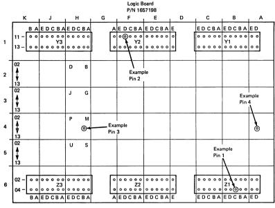
Logic Board Pin Layout Pin Side
