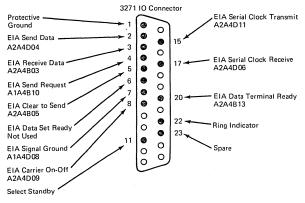
25-Pin Connector Mounted on 3271
