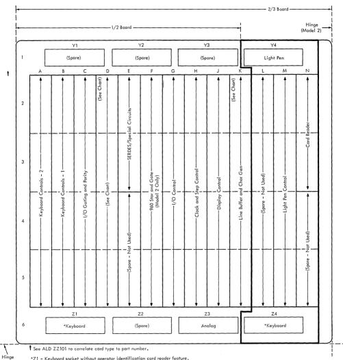
\*Z1 - Keyboard socket without operator identification card reader feature. Z4 - Keyboard socket with operator identification card reader feature.
