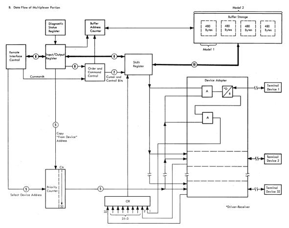
Figure 2-1 (Part 2 of 4), 3271 CU Functional Block Diagram
