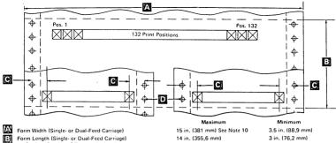
Carriage Spacing-6 lines per inch only. with the left tractor in leftmost position.
