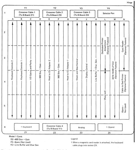
Figure 4-6. 3275 A-Gate Card Layout by Function (Display)
