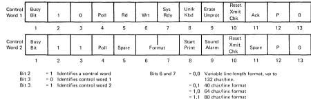
*Note:* Either or both control words may be transmitted to a selected Display Station or Printer.
