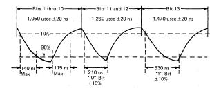
The pulse amplitude, as referenced to dc return (outer conductor of coaxial cable), will be as follows for a control unit or device:
