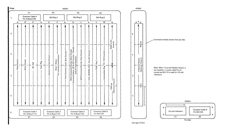
Figure 8-5. 3275 Model 11 and 12 Card Layout by Function - B-Gate
