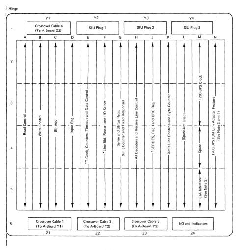
Figure 4-10. 3275 B-Gate Card Layout by Function (Dial)
