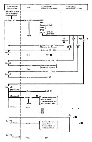
Figure 1-45 (Part 1 of 2). Write-Type and Control-Type Commands, Sequence/Response Diagram
