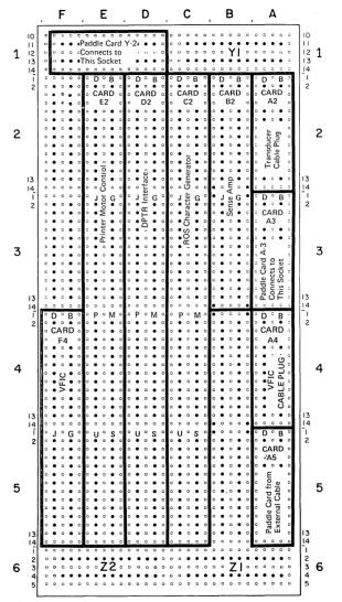
Figure 6-7. 3284/3286 Model 3 A-Gate Card Layout by Function - VFIC
