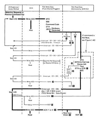
Figure 1-46 (Part 1 of 2). Read-Type Command, Sequence/Response Diagram
