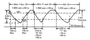
Bit timings from the device to the control unit will meet the same requirements as from control unit to device except for bit rate. The bit rate from the device will be 630 ns (min) to 1.050usec (max) per bit. The minimum duration of the Up level, after crossing the 10% point going in the positive direction for a 1 or 0 bit until the start of the next consecutive bit, will be 30 ns.
