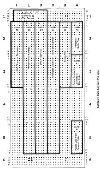
Figure 6-6. 3284/3286 Model 3 A-Gate Card Layout by Function - Dual Case
