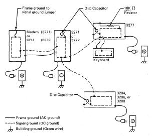
Figure 1-2. 3270 System Grounding
