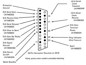
Note: Signals from data set to 3275 measure +3V to +25V for up level and 3V to -25V for down level. Signals to data set for 3275 measure +3V to +8V for up level and 3V to -12V for down level.
