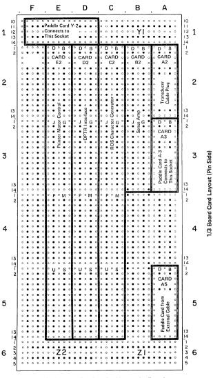
Figure 6-5, 3284/3286 Model 3 A-Gate Card Layout by Function
