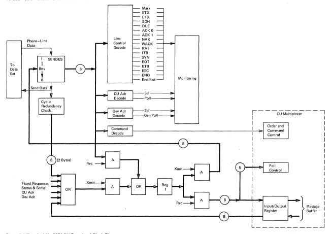
Figure 2-1 (Part 1 of 4). 3271 CU Functional Block Diagram
