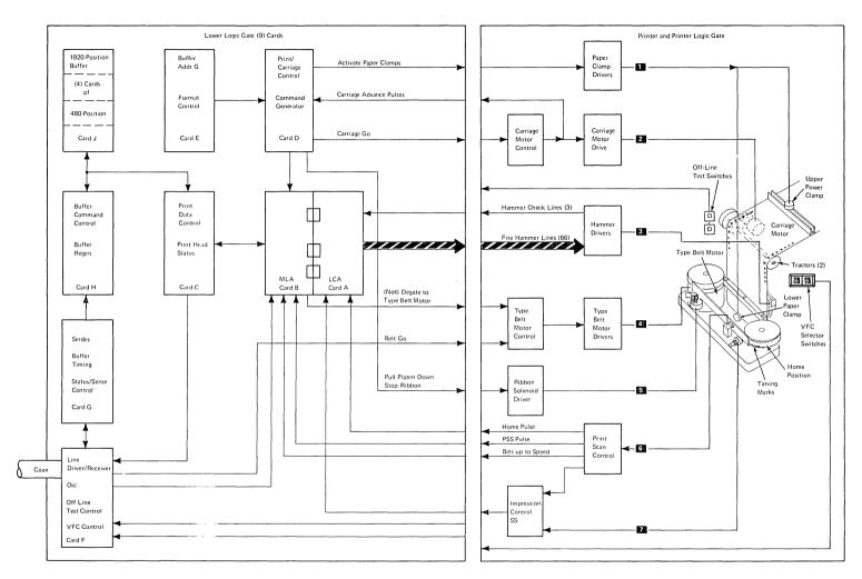
Figure 7-1. 3288 Block Diagram
