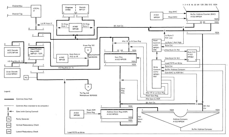
Figure 3-1. 3272 Control Unit Data Flow
