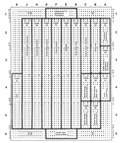
Figure 6-4. 3284/3286 Model 1 and 2 A-Gate Card Layout by Function - VFIC
