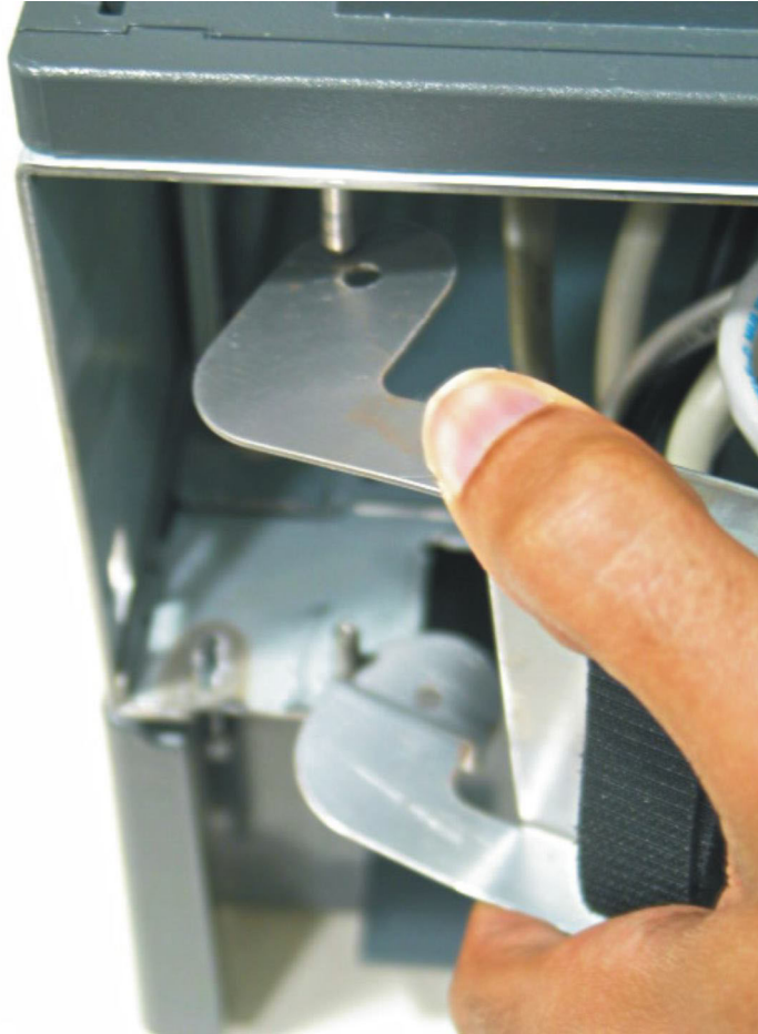
Figure 60. Attaching the cable guide arm assembly
