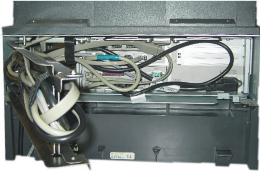
Figure 62. Cable assembly arm with cables securely in place
