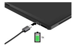
Note: To maximize the life of the battery, use the battery until the charge is depleted and recharge the battery completely before using it. Once the battery is fully charged, it must discharge to 94% or lower before it will be allowed to recharge again.
